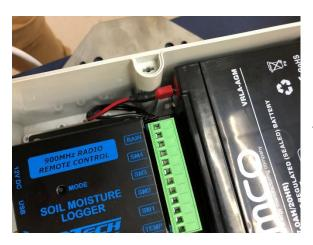
Open the Remote solar station. The soil moisture wiring as been done in the factory, all that is required it to connect the positive battery terminal.
