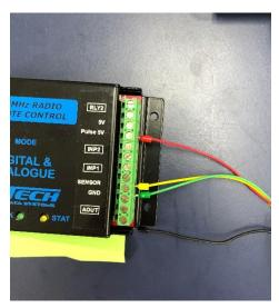
The tank level sensor comes prewired from factory but may need unplugging for installation in the tank. The table and the picture below show how the sensor is wired into the ITU. When installing sensor in the tank make sure the cable isn't bent too much as this could damage it.
