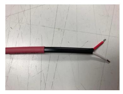
Strip the ends on the Soil temperature Probe (marked red) wire to expose around 5mm of the copper. As shown in the picture
