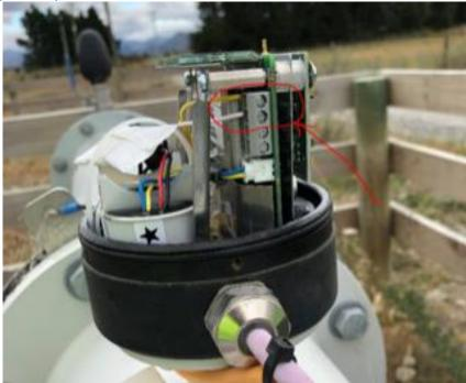
The yellow wires goes to pin 58 of Output A. The White wire to pin 57. With the pullup at the ITU end negative pulse logic will be used.
